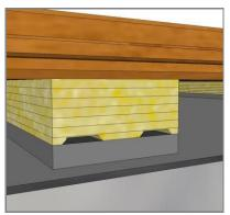
KTL SPORT MULTIFLEX ADVANCED V2 is an area-elastic sports floor, based on 22mm solid hardwood 2-strip parquet boards, nailed to a resilient 1-layer batten system, installed floating on levelled concrete or wooden based subfloor. Total construction height incl. floorboard is 52mm.
